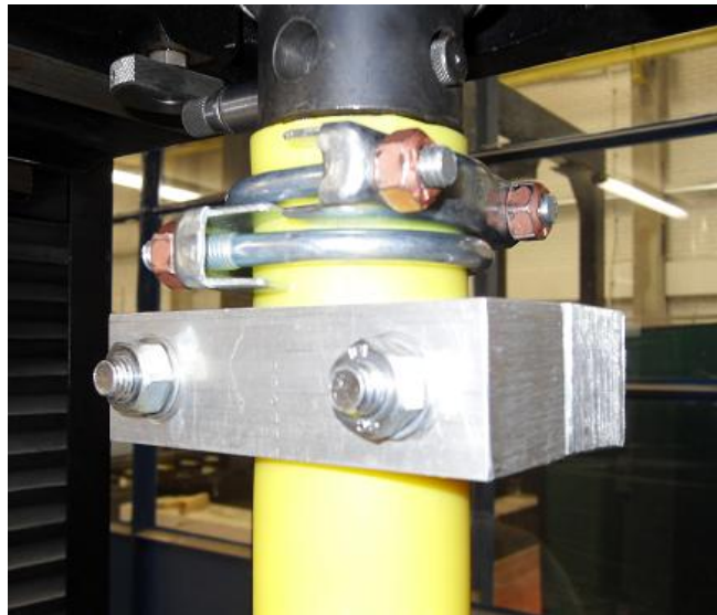
Figure 28. End restraint design (two pipe clamps and wide clamp)
