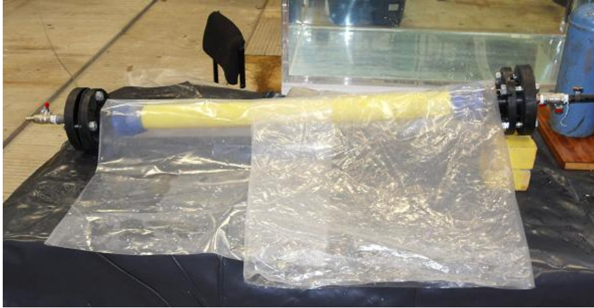
Figure 26. Plastic sheeting protection from testing rig
