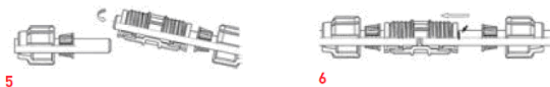
Figure 8. Stages 5&6 compression coupler joining procedure (George Fischer 2010b)
