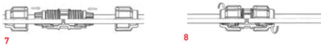
Figure 9. Stages 7&8 compression coupler joining procedure (George Fischer 2010b)
