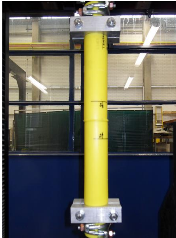
Figure 39. Manual butt fusion jointed test piece necking during tensile strength test
