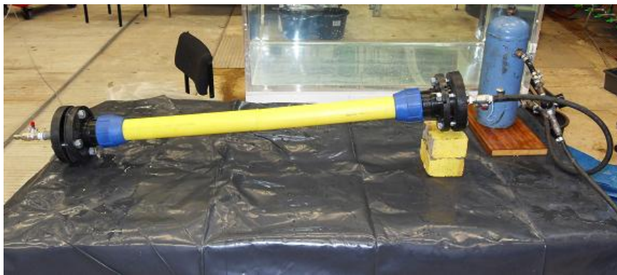
Figure 24. Hydrostatic pressure testing rig
