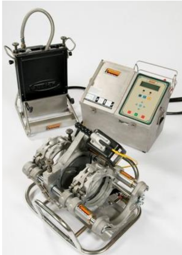
Figure 2. Automatic Butt Fusion Machine (Fusion Provida 2010)
